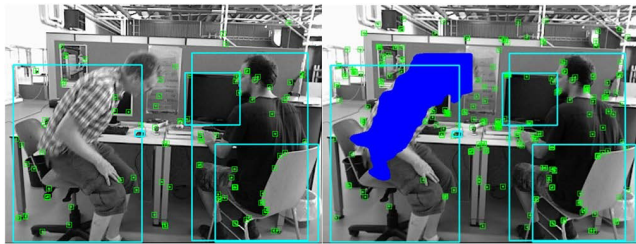
FIGURE 8. The value of the optical flow vector is used to determine whether the pixel is moving to avoid rejecting static features on dynamic objects. Then, use dynamic pixel to build an optical flow mask, and remove all dynamic feature points in the mask.
