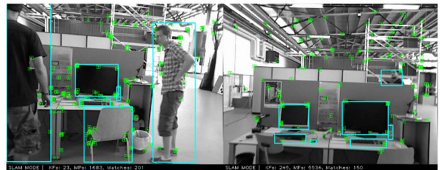
FIGURE 3. In the semantic thread, YOLOv5s perform semantic box extraction on objects such as pedestrians, books, tables, and chairs in key frames. The semantic box contains almost all objects that have the possibility of moving.
