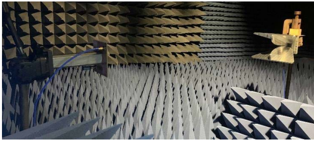
FIGURE 11. Measurement setup to analyze radiated characteristics of the MF in the far field.
