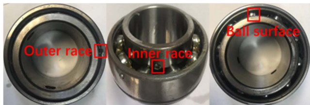
FIGURE 9. Locations and shapes of bearing defects.
