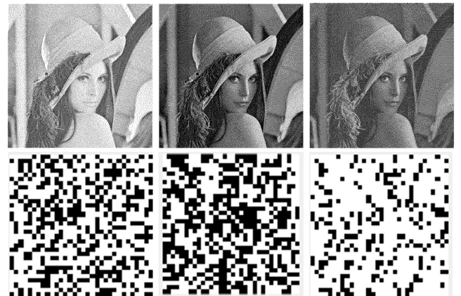
FIGURE 18. First row shows fragile watermarks extracted from Lenna's dual watermarked image in the absence of an attack. Here, the left-most impression is of the fragile watermark extracted from the red colour channel. The middle and the right-most images are the fragile watermarks extracted from the green and blue channels, respectively. In contrast, the second row shows fragile watermarks extracted from Lenna's dual watermarked image after it's been exposed to the median filtering attack. Best viewed when zoomed-in.
