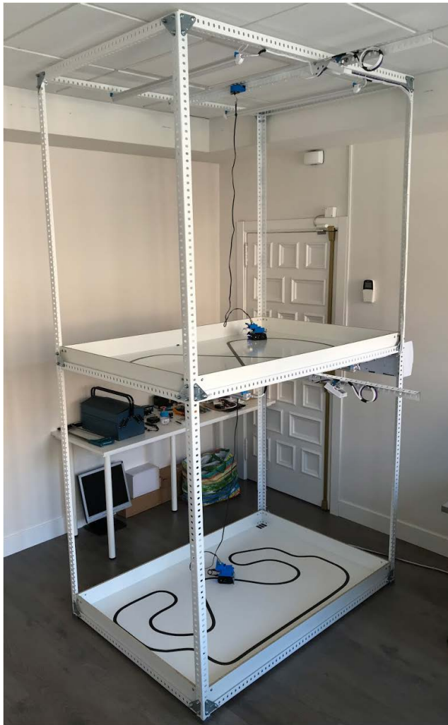
FIGURE 4. Supporting structure for a couple of LabsLand's Arduino Robot experimentation instances. The tracked robot, which is controlled by the user's code, can be moved over the entire surface of each rectangular tray.
