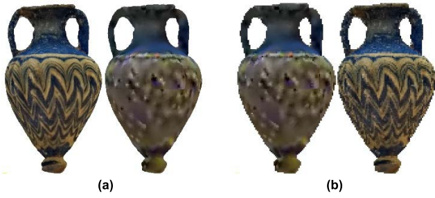
FIGURE 3. Amphoriskos PC decoded with G-PCC in Octree geometry coding mode and Lifting color coding mode at the lowest rate: (a) PCs obtained for the reference geometry with the reference (left) and decoded color, after recoloring (right); (b) PCs obtained for the decoded geometry with the decoded color (left) and reference color, after recoloring (right).
