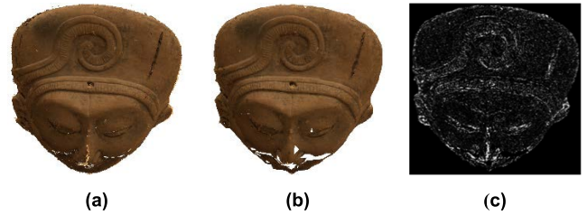
FIGURE 2. Egyptian Mask PC projected from front view: (a) Reference PC; (b) Decoded G-PCC geometry for lowest geometry rate, recolored with the original color; (c) Residual image between (a) and (b) after enhancement.
