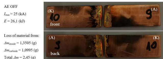
FIGURE 9. Erosion of the copper electrode material as a result of the high-current electric arc action.
