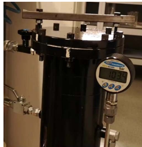
FIGURE 10. Hyperbaric pressure testing rig.
