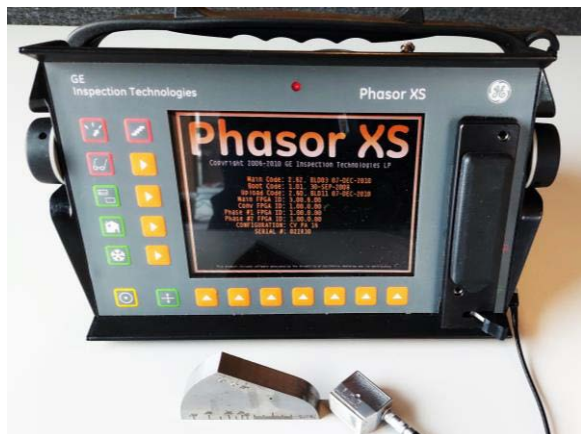
FIGURE 11. GE Phasor XS and the probe used in the non-destructive testing.
