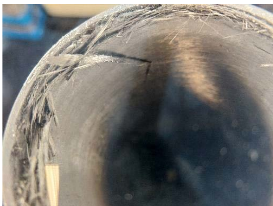
FIGURE 12. Failure resulting from the implosion of the tube.
