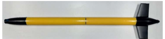
FIGURE 1. An assembly of the underwater vehicle, showing the designed pressure hull in yellow and the fairings in black.
