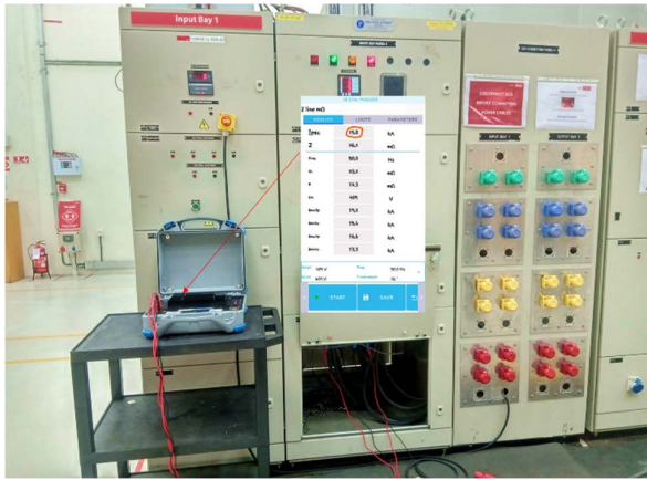
FIGURE 6. Grid impedance measurement set-up (METREL 3144).
