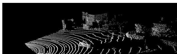
(c) Point cloud in fog condition.
