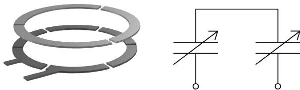
FIGURE 2. Arrangement of the electrodes of the gap-sensing capacitors on the upper and lower substrates of the FPI. Only two of the six bonding areas are drawn. On the right is a schematic representation of the resulting series connection of one pair of capacitors. In the following schematics, the series connection is drawn as one variable capacitor, C_{fpi} .
