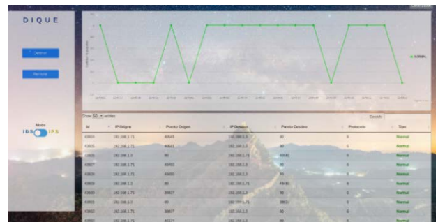
FIGURE 32. View from Dique of a TCP flood attack.
