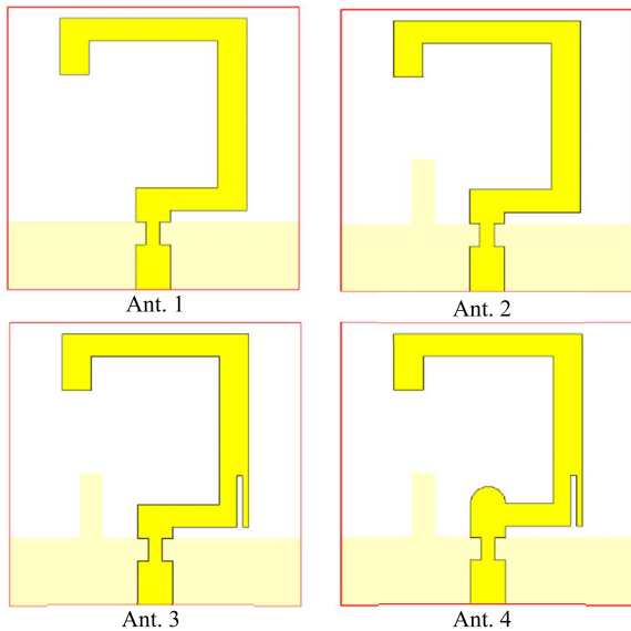
FIGURE 2. The design procedure of the proposed antenna.
