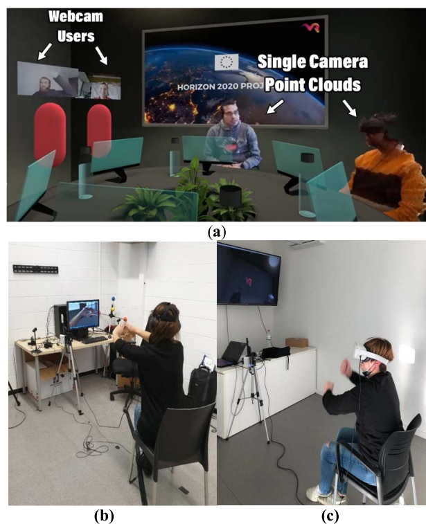
FIGURE 1. Holomeeting scenarios using the social VR platform: a) holomeeting with four users, two of them represented as volumetric point clouds; b) and c) evaluation setup, with one RGB-D camera, one desktop or laptop, and one head-mounted display (HMD).
