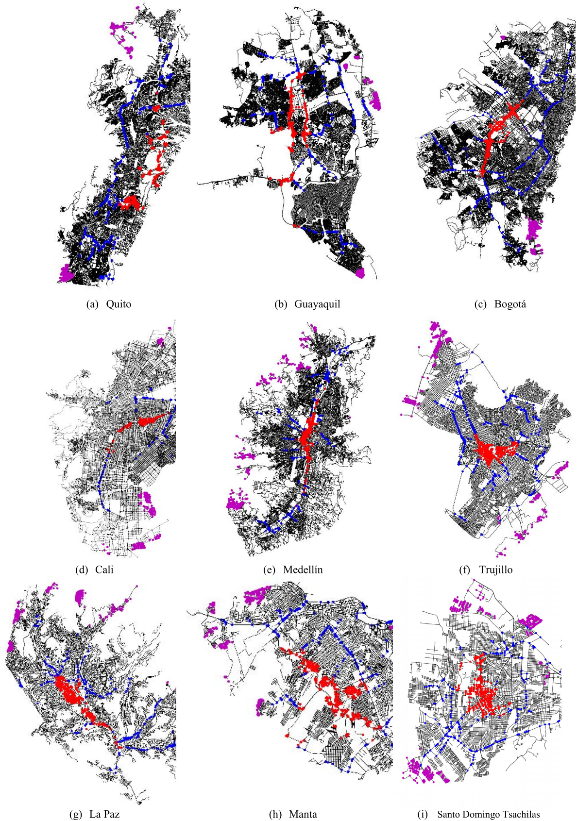
FIGURE 10. Fusion of indicators for BC, CC, and eccentricity of urban networks. Fusion of indicators for BC (nodes blue), CC (nodes red), and eccentricity (nodes purple) of urban networks.
