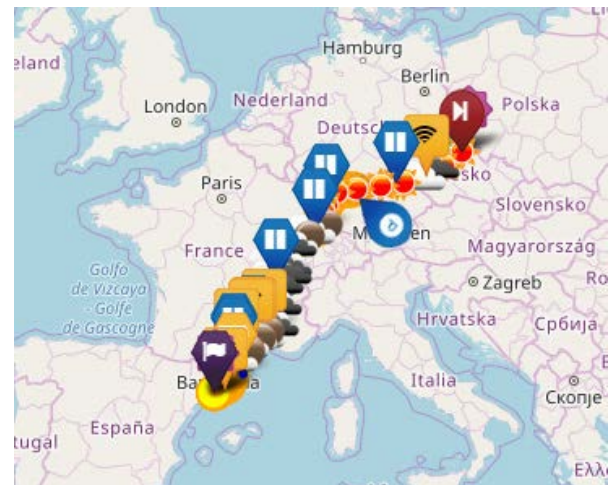
FIGURE 8. Details of track recommended by Smart Driving Service. Blue icons represent stops and yellow icons are the recommended speed values. The start and end of the route and weather forecasts are plotted.
