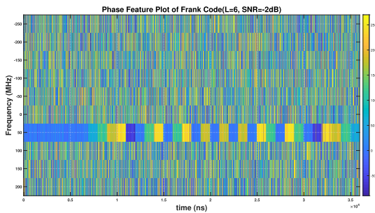
FIGURE 5. Phase Feature Plot of Frank Code (L=6, SNR=-2 dB).
