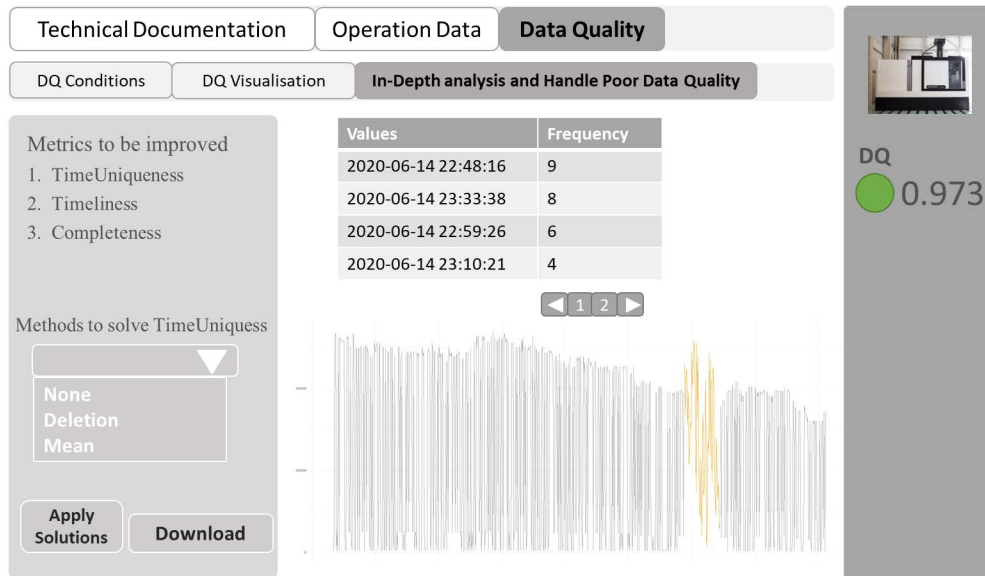
FIGURE 18. Interactive dashboard in which to choose low quality resolution methods and inspect the results.
