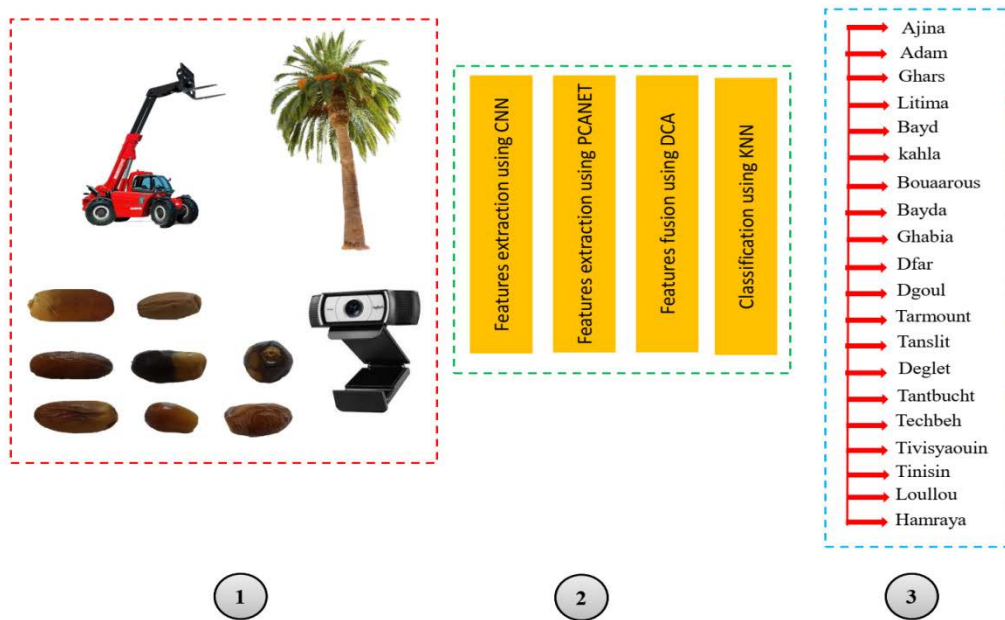
FIGURE 3. The pipeline of the date fruit sorting process: 1) Date fruit harvesting and image acquisition, 2) features extraction and classification, and 3) different classification outcomes.
