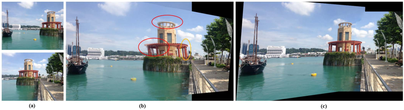
FIGURE 1. Comparison of the results of a representative spatially varying warping method (APAP) [4] and our method. (a): The input image [13]. (b): The stitching results of APAP, which exhibit not only visual distortion but also obvious ghosting. (c): The stitching result of our approach, in which the distortion and ghosting are eliminated.
