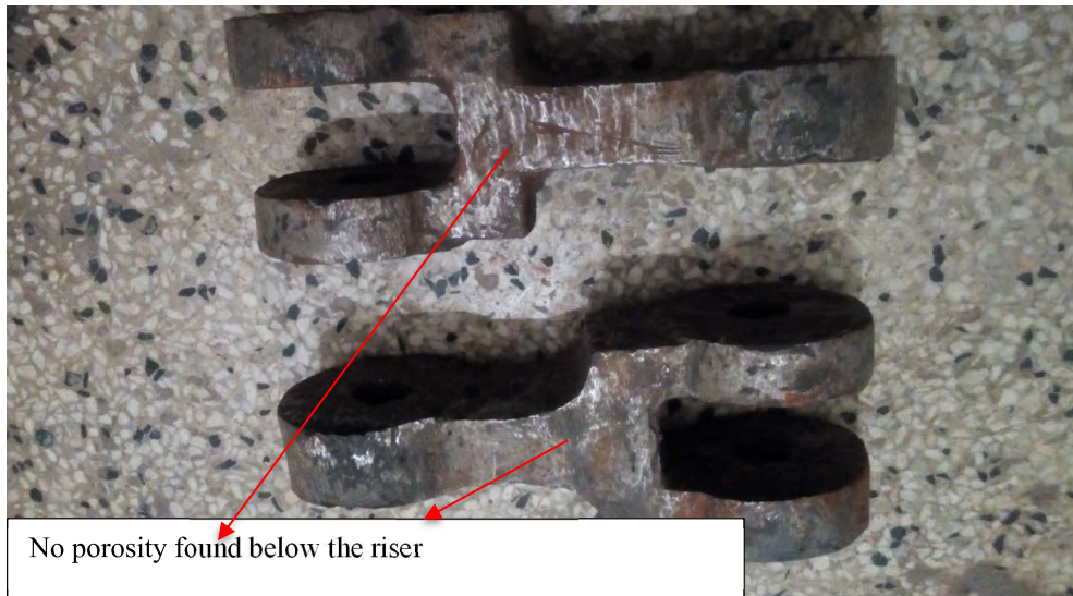
FIGURE 12. Y-chain link without porosity.
