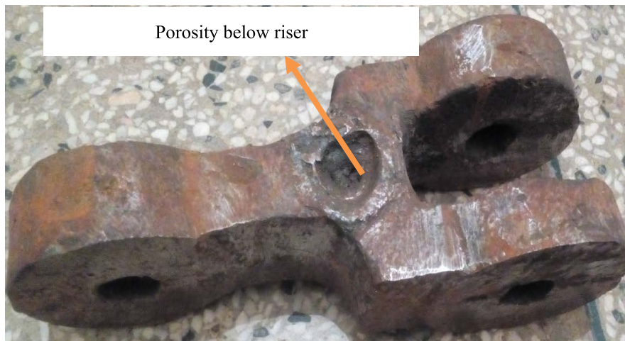
FIGURE 5. Y-chain link with porosity.
