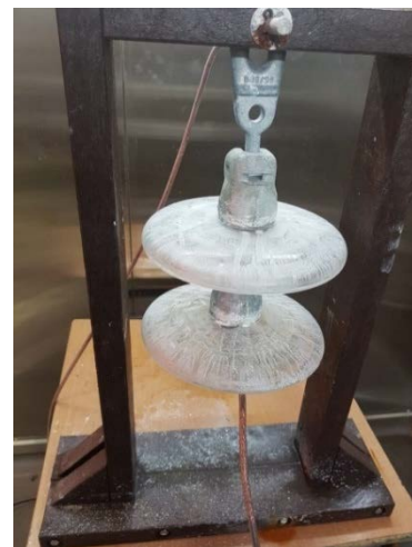
FIGURE 3. Polluted insulator string.
