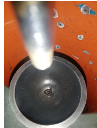
FIGURE 7. Particles in bowl electrode.
