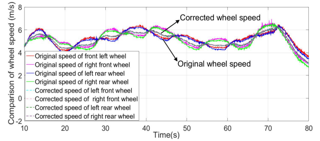
FIGURE 2. Comparison of wheel speeds before and after correction.
