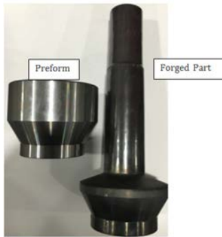
FIGURE 9. Preform and forged part with a Factory Acceptance Trial (FAT) geometry, which is used to test and demonstrate radial forging capability.
