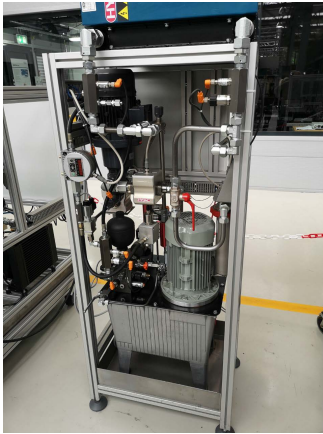
FIGURE 6. Hydraulic system test rig for condition monitoring at ZeMA, Germany.
