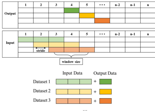
FIGURE 6. Learning dataset construction method of periodic data by using time sliding window (e.g., sinusoidal signal).
