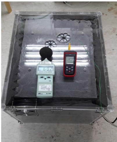
FIGURE 3. Acrylic mask perforates the fan and measures the temperature inside the mask.
