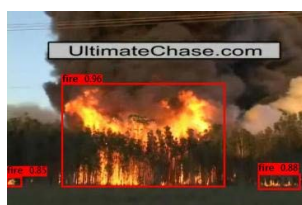
FIGURE 8. Some video-based fire detection results with improved Yolo-v4 algorithm (a) Video 1, (b) Video 2, (c) Video 3, (d) Video 4.
