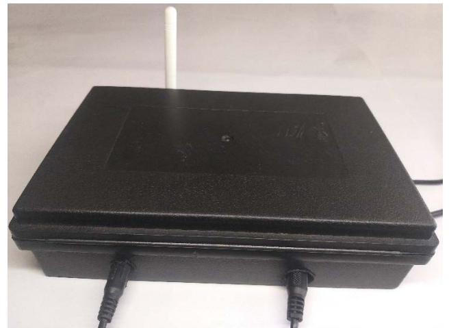
FIGURE 14. An EEMD encapsulated in a waterproof protective casing.
