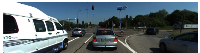
FIGURE 14. Start and stop moment with multiple moving vehicles in the surrounding area. As the other vehicles move, while the sensing vehicle is stationary, they cause a false sensation of motion [3].
