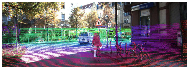
FIGURE 8. Visualization of depth enhanced images as in DV-LOAM's front-end odometry module. This Figure illustrates the point cloud projection into the respective camera frame. Different colors represent different levels of depth.
