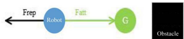
FIGURE 8. Local minimum problem with target point between obstacle and robot.
