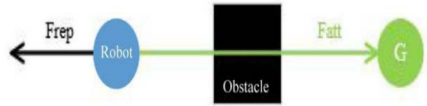
FIGURE 7. Local minimum problem of obstacles between robot and target point.
