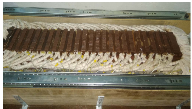
FIGURE 9. Prototype SLIM stator with sliding support for secondary sheet.
