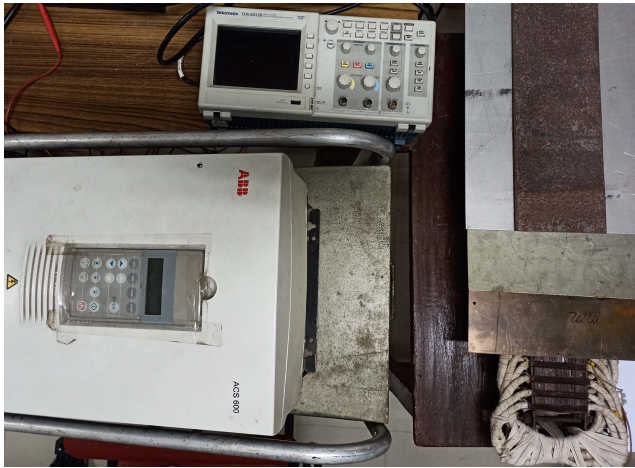
FIGURE 10. Setup for testing of the prototype SLIM.
