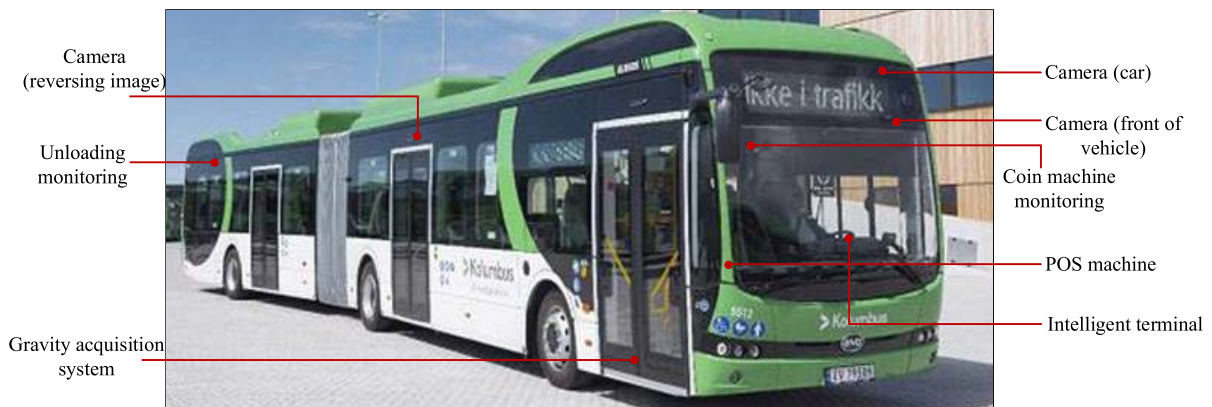
FIGURE 10. 3D display processing of information acquisition equipment in shared vehicle system.
