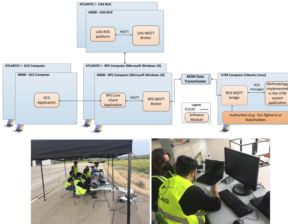
FIGURE 9. Setup for the experiments. On top, an view of the interfaces between the components run on each computer. The computers running the RPS for the two UAS and the UTM system were communicated through the internet via the MQTT protocol. At the bottom, pictures of the UAS Ground Control Station (left) and the UTM computer (right).
