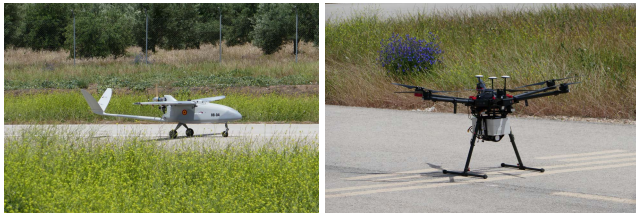
FIGURE 8. The Atlantic I (left) and DJI M600 Pro (right) UAS used in the field experiments.
