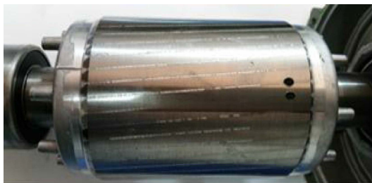
FIGURE 3. Broken rotor bars faults cause speed oscillations in the rotor, leading to premature wear of bearings and other components [28]. The condition can be detected using MCSA and can be artificially generated by drilling holes in rotor bars.
