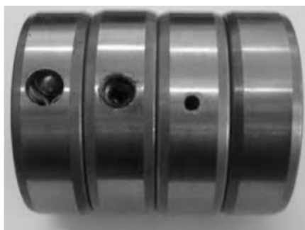
FIGURE 4. In the presence of a bearing fault, the rolling elements (balls) pass over the defect area periodically, producing impulses with a certain frequency, which can be detected by MCSA [29]. The condition can be artificially generated by drilling holes of various diameter.
