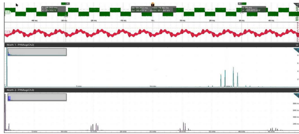
FIGURE 43. Current THD and voltage THD generation.
