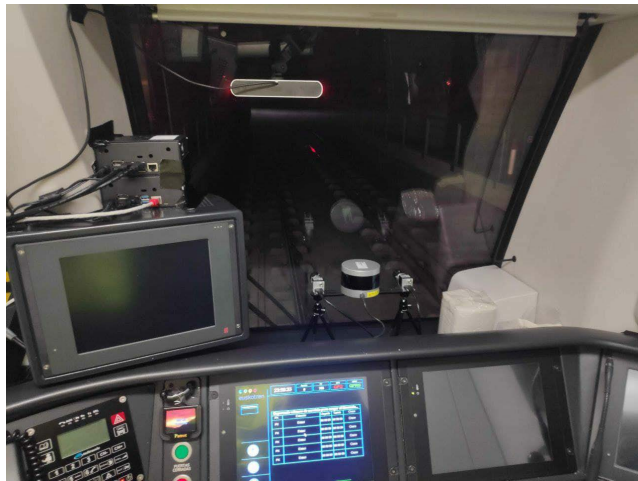
FIGURE 2. Camera setup for CAF dataset, placed in the cabin of a train moving through an underground urban railway scenario.
