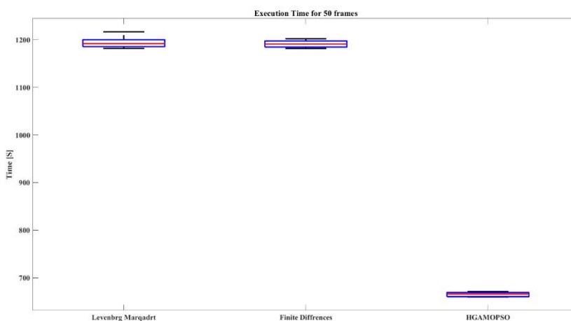
FIGURE 15. The total execution time of algorithms as boxplot: the proposed algorithm is faster and consumes approximately 56% of the time consumed by the levenberg algorithm and approximately 58% of the time of finite defrence.
