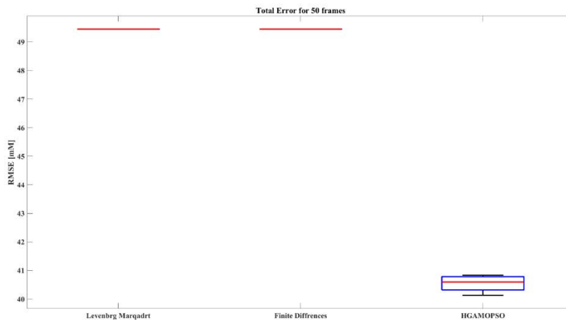
FIGURE 14. The RMSE value for the entire trajectory as a boxplot: The highest error value for GAMOPSO is less than 20% of the minimum error value of the benchmark algorithms.
