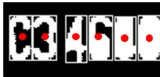
FIGURE 10. The initial character locations detected and the adaptive labeling is carried out using the centers of bounding boxes.
