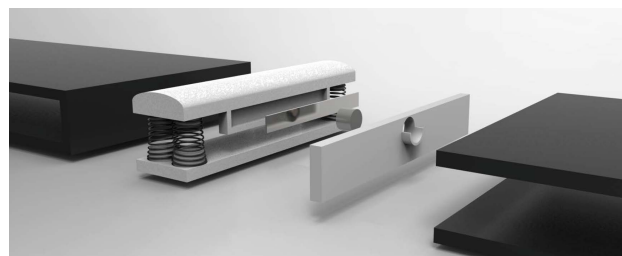
FIGURE 4. 3D CAD model of the speed bump prototype in a modular design.
