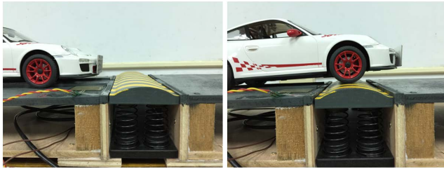
FIGURE 13. The miniature road bump created by 3D printing.
