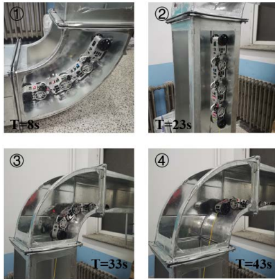
FIGURE 21. Wall climbing experiment.
