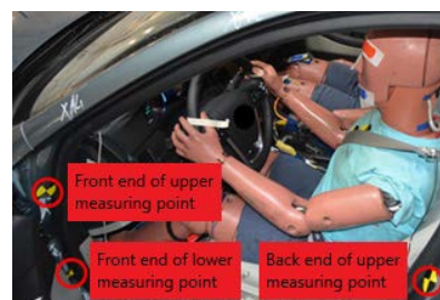
FIGURE 20. Position of door deformation measurement point.
