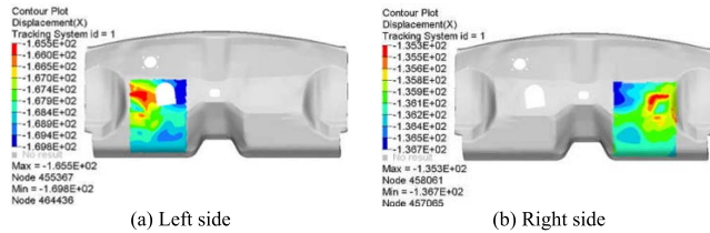
FIGURE 21. Cloud map of foot pedal intrusion displacement.
