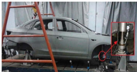
FIGURE 9. Torsion stiffness test of BIW.
