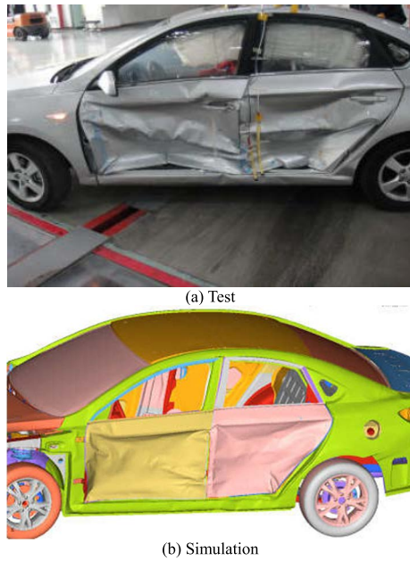
FIGURE 24. Deformation pattern of the car in side impact.
