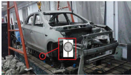
FIGURE 5. Schematic diagram of bending stiffness test conditions and measuring points of the BIW.
