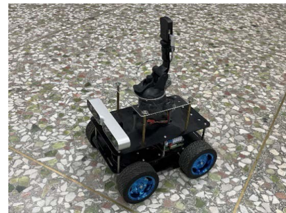
FIGURE 2. A 4W skid-steering mobile robot for experiment.
