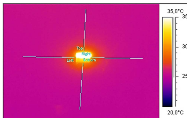
FIGURE 20. Thermal camera image of the laser scribing process. The bright square ( 4 \times 4 mm) in the middle is the laser processed area, and the brighter line inside is the laser spot moving sideways. Temperature was measured along the four lines, which were added to the video after the processing.
