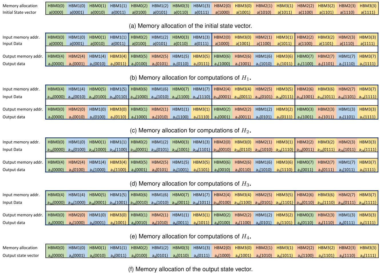
FIGURE 8. Proposed memory allocation of Hadamard gates. After each Hadamard gate computation, the output data are used as the inputs of the controlled phase-shift gate computation. Since each output of controlled phase-shift gate replaces its inputs, the memory allocation remains the same. The inputs of H2, H3 and H4 are the data after the controlled phase-shift gate computation.
