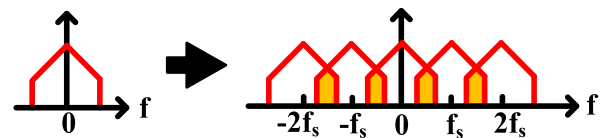
FIGURE 3. Phenomenon of aliasing signals.
