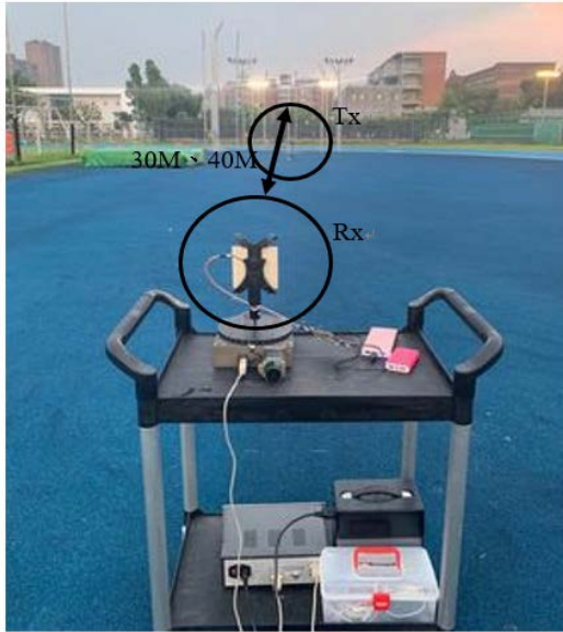
FIGURE 5. Measurement setup at NTU campus, where Tx is WiFi AP and Rx is DoA module mounted on a turn table and located 30 or 40 meters in front of WiFi AP.
