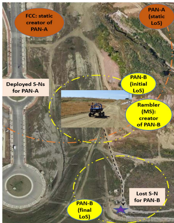
FIGURE 7. PANs of the zigbee H-WSN. The mobile coordinator node embarked on Rambler generates a dynamic coverage radius.
