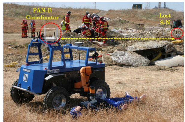
FIGURE 6. Rambler carrying the mobile C-N (PAN-B coordinator) assisting the dummy-victim. At the same time, it is providing coverage to the lost Bluetooth S-N. Behind the robot, human agents attend to buried victims.
