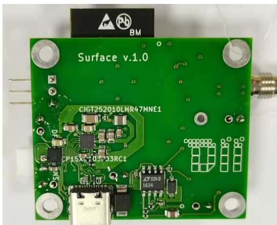
FIGURE 9. Top and bottom view of the purposely designed board.
