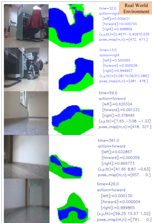
FIGURE 8. Experimental results in the real world. Each experiment conducted 500 time steps (one time step is about 1.5 seconds, which is the processing time of the TVENet on the robot.) This figure shows five time steps in different experiments.
