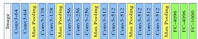
FIGURE 2. The architecture of VGG16 network.
